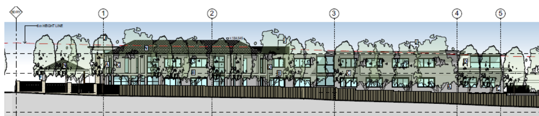
Figure 2 – Section showing the 3 storey element located through central portion of the development with the green line representing existing ground level
