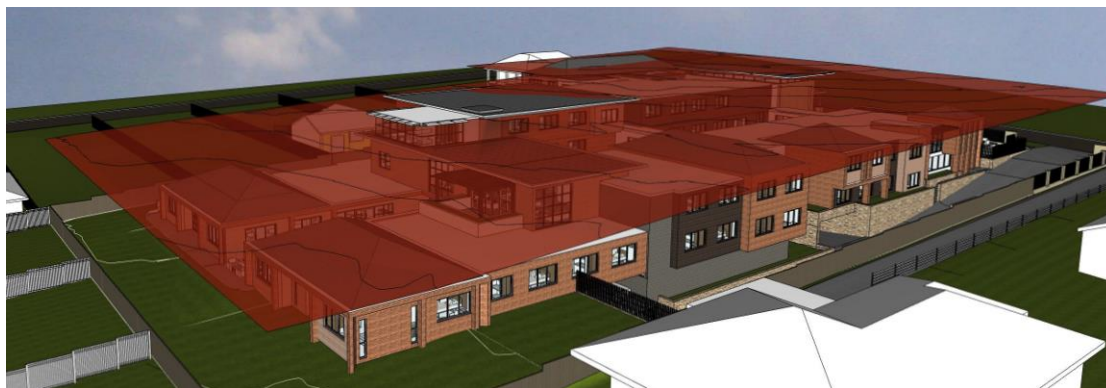
Figure 10 – Height blanket diagram showing strict compliance with the 8 metre ceiling height standard.
