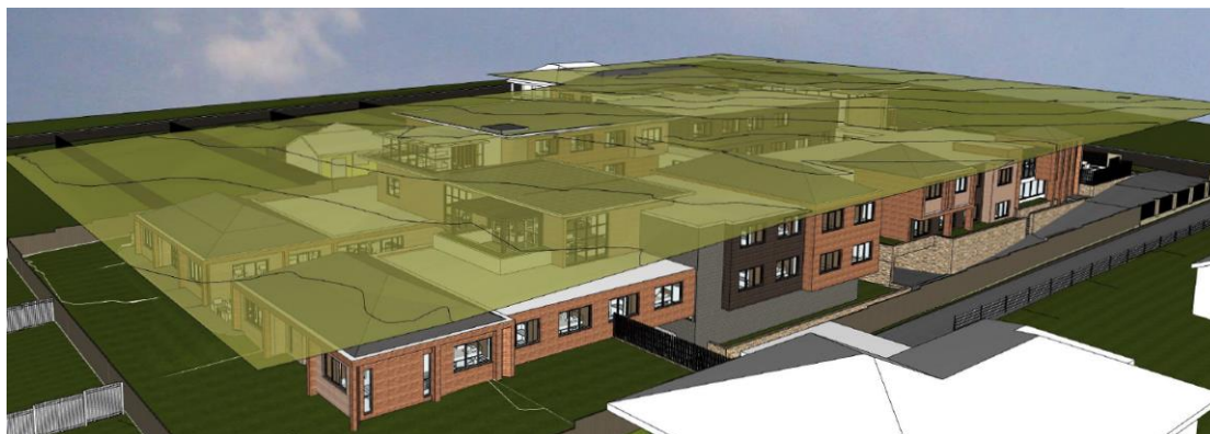
Figure 9 – height blanket diagram showing minor breaches of the 8.5 metre height standard.
